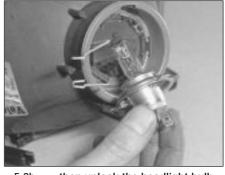
5.2b ... then unlock the headlight bulb retaining spring and withdraw the bulb
